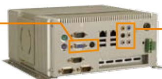
TV-out Port • Supports S-Video, Component and Composite video signal output • Component output up to 1080i/1080p
